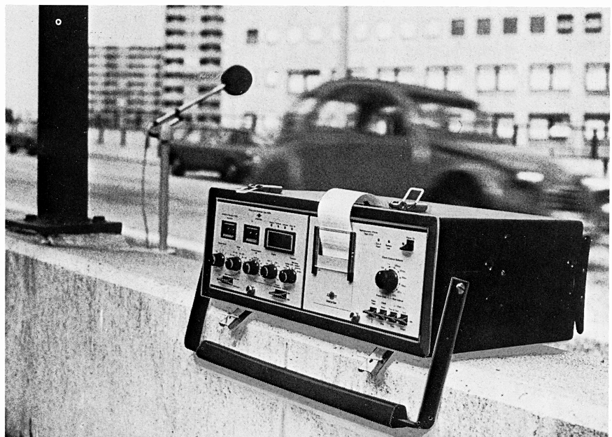
Fig.6. The Alphanumeric Printer Type 2312 and the Noise Level Analyzer Type 4426 in use for on-site measurement and statistical analysis of traffic noise
